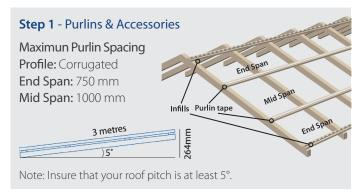
Never walk directly on COOL TOP, or any other Polycarbonate/PVC sheets. Use a board placed across at least 3 purlins to spread the load.
